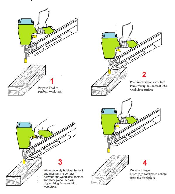
With this type of actuation, additional fasteners can be fired provided the <u>trigger is released</u> and the <u>workpiece contact remains depressed</u> and is in contact with the workpiece surface **or** provided <u>both</u> <u>the trigger and the workpiece contact can be disengaged</u> and reengaged in the same sequence.
