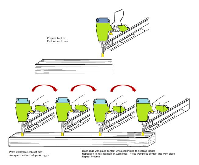
In this process shown above, the trigger is depressed and held, as the workpiece contact is bumped from point to point a fastener is fired from the tool.
