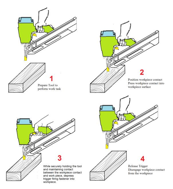
With this type of actuation, additional fasteners can be fired provided the <u>trigger is released</u> and the <u>workpiece contact remains depressed</u> and is in contact with the workpiece surface **or** provided <u>both</u> the trigger and the workpiece contact can be disengaged and reengaged in the same sequence.
