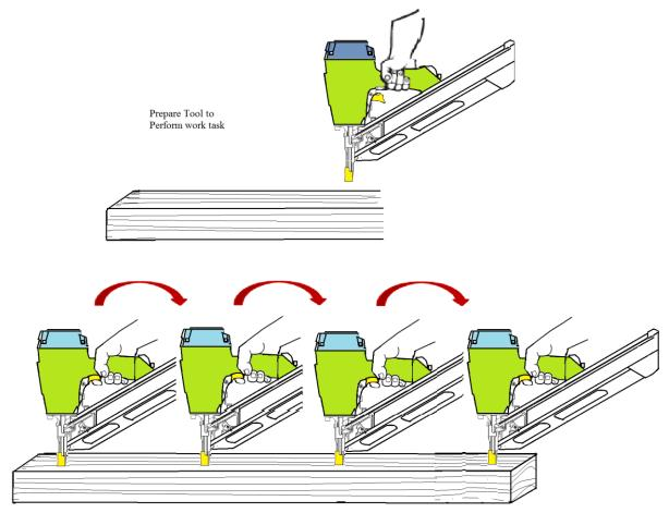
Press workpiece contact into workpiece surface - depress trigger Disengage workpiece contact while continuing to depress trigger Reposition to next location on workpiece - Press workpiece contact into work piece Repeat Process
