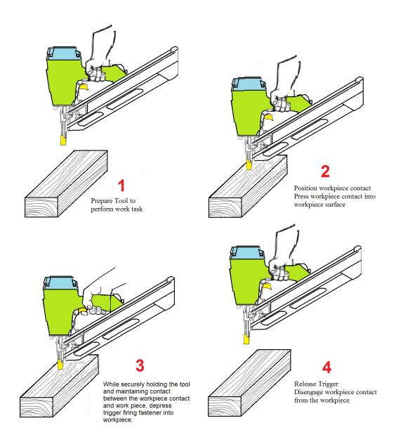
With this type of actuation, additional fasteners can only be fired after the <u>trigger is released</u> and the <u>workpiece contact is disengaged</u> from the workpiece surface.
